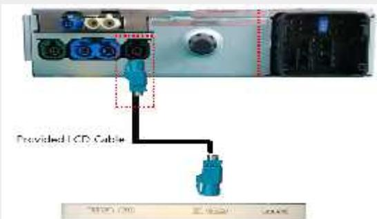
Connect the interface LVDS cable with the NAC computer (black connector) and the other side with the interface input "OEM IN".
