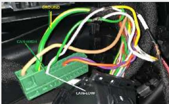
Connect above open wires with original cable as above
