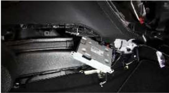
**3008:** You can find the radio module behind the gear shift. You can access the computer by removing the side panel.
