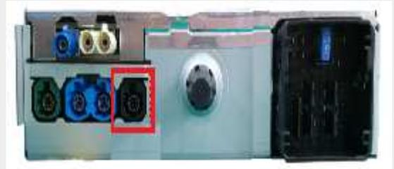
Disconnect the original black fakra LVDS cable from the computer and Connect the original LCD cable with the interface input "OEM-OUT".
