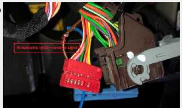
Big brown connector on fuse box pin #50 is for reverse gear signal (12V).
