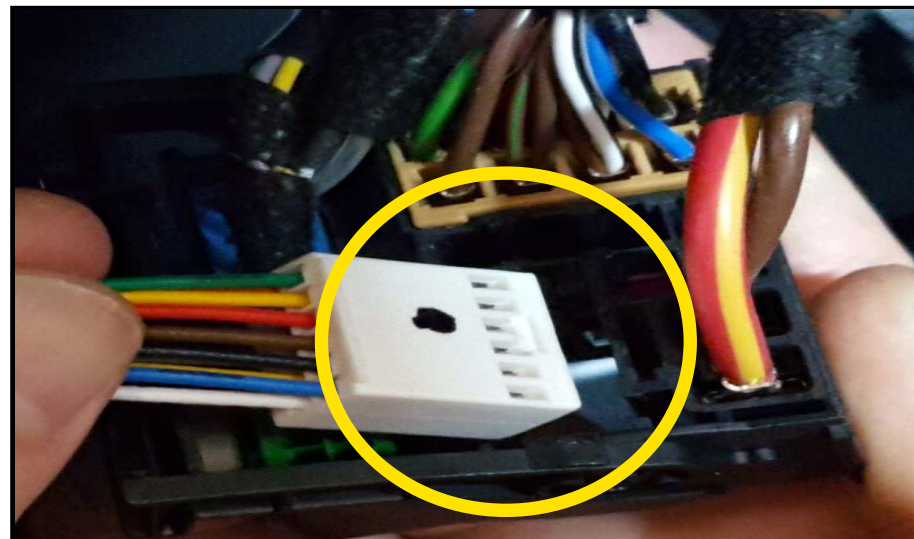
2. PLEASE INSERT CONNECTOR OF INTERFACE WITH THE BLACK POINT IN THE UPWARD DIRECTION.
