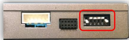
**Note:** Remove power to the unit prior to making adjustments to the dip switches
