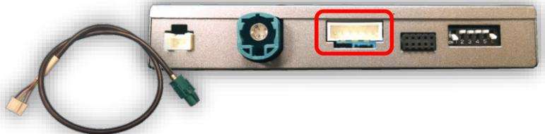
5. Connect the free end of the provided **LVDS Video Cable** (green) back to the factory radio at the bright **GREEN** cluster LCD port.
