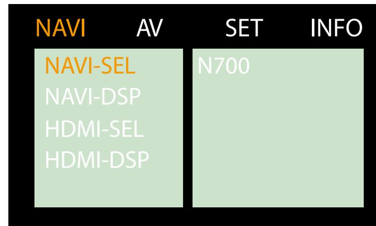
Please press "OK" button 4 times and press "POWER" button once to enter into our OSD menu by remote controller and select HD-G2/N700 after installing our interface and our Android box by HDMI cable.
