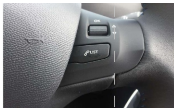
18. While the AUX input setting completes, press " LIST" on steering wheel button for 3 seconds to enter our navigation interface
