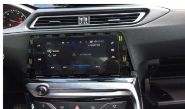
3. Take out the screen frame, and remove the screws at the right corner and left corner of the screen
