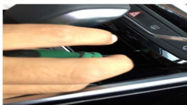
4. Take out the rubber mat beneath air condition button
