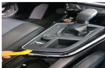
5. Detach the decoration panel around the gear shift lever
