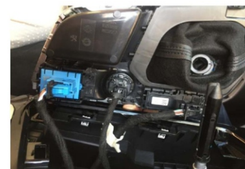
7. Take out the handle of the gear shift lever , and unplug the cable
