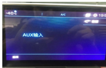
18. While the AUX input setting completes, press " LIST" on steering wheel button for 3 seconds to enter our navigation interface
