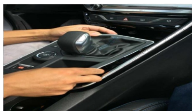
6. take out the panel carefully, and pay attention to the cables
