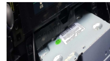
10. Take out the OEM head unit and OEM screen
