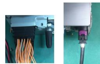
9. Take out the panel beneath gear shift lever, and detach the screw of DVD
